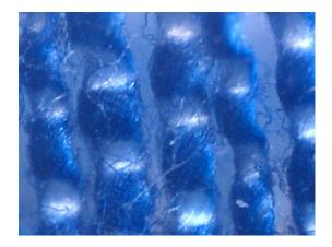
After the fibres are teased out, poor dyeing is obvious where the fibres cross.
